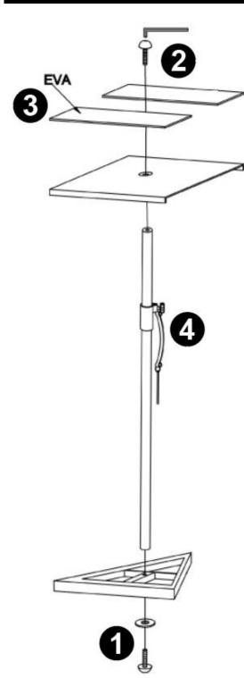
**Step 1:** Tightening the tube and base with screw and washer.
