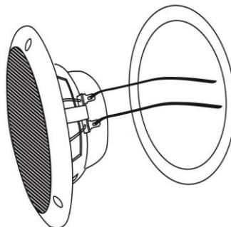
3. Insert the speaker in the hole and screw down each of the screws.
